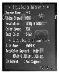
Press  $[M/\leftarrow]$  to check the input/output device information and software version.
